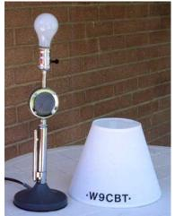
Get a length of the type of threaded brass tubing used in lamps, it's about 3/8" in diameter. The tubing is cut to length after you locate a light bulb socket with a switch. I wanted a chrome finish light socket -- that is easier said than done. None of the major DIY outlets carry a silver-colored socket. I finally located one at a lamp store. A black plastic one would work fine, too.
