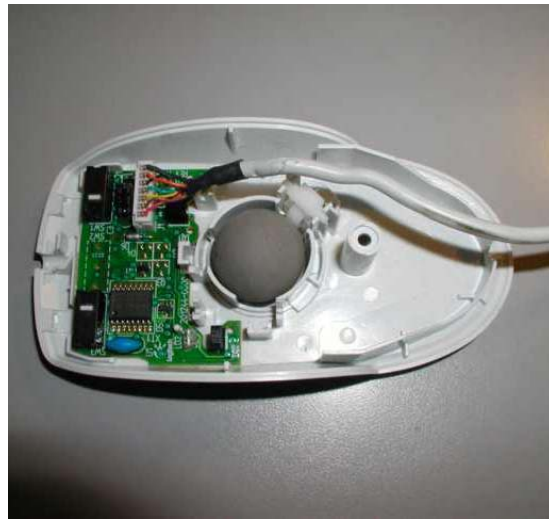
Under the Hood — Note Cable Reversed
